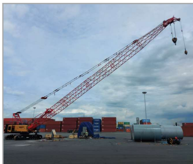
CẦN TRỤC BÁNH XÍCH SANY SCC550A - 55 T CRAWLER CRANE OF SANY SCC550A - 55 TONS
