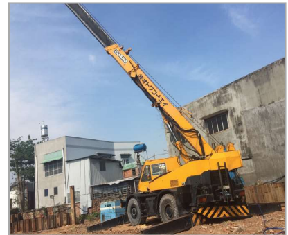
CẦN TRỤC BÁNH LỐP TANADO TR250 - 25T WHEEL-MOUNTED CRANE OF TANADO TR250 - 25 TONS
